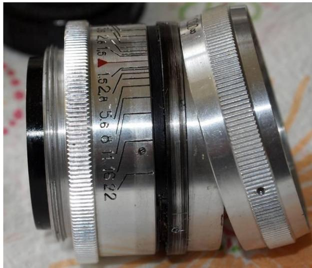
The focus ring comes off with three set screws. Keep the individual set screws in order, remember the starting position and put the screws in different bins of a tray. Use a screwdriver that matches well with the slot, the screws break easily. The focus ring slides forward to reveal the screws holding the helical into the mount. Note the taps under the
