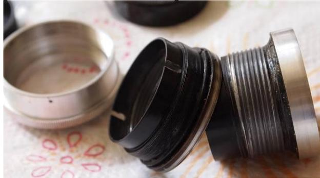
With the guide pins out, the inner helical unscrews. The grease is usually dry, and needs to be removed completely. Save those old tooth brushes and dip them in alcohol or lighter fluid. The inner helical can be dropped in an ultrasonic cleaner if you have one.
