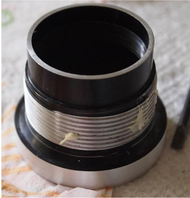
Use a little grease on the inner helical. Some helicals have more play than others; excess grease will work forward as you screw it in. Wipe off that excess.
