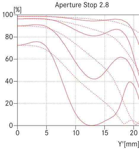
At aperture 2.8 the overall contrast is visibly improved as is the quality in the outer zones of the image. The very fine detail however has a softer definition.
