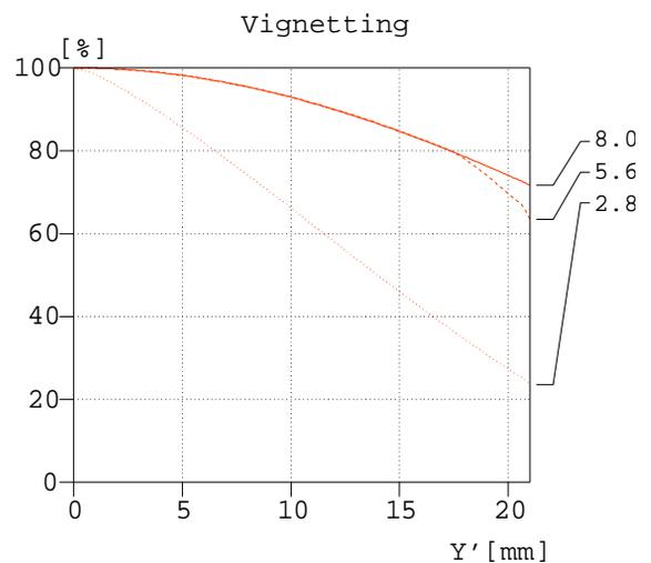
Vignetting is acceptable with 1.8 stops and will not be disturbing in most cases.
