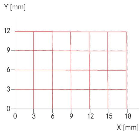
The distortion of the Summilux-R is visible with 2%.
