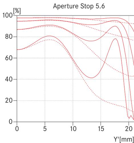
At apertures 4 and 5.6 the optimum is reached. The graphs of the 20 lp/mm and the 40 lp/mm are a bit wavy. At an image height of 12mm there is a weaker zone, the result of aberration compensation. The improvement beyond an image height of 18mm is the influence of the vignetting. The vignetting is acceptable with two stops and will only be detected at the edge of the negative when larger areas with the same brightness are recorded.
