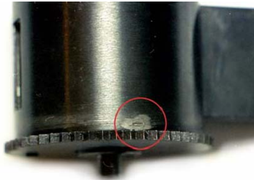
Fig. 7: screw to open the lens turret
