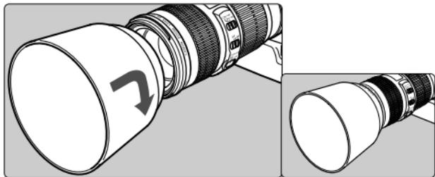
The ET-74 hood can keep unwanted light out of the lens, and also protects the front of the lens from rain, snow, and dust.
