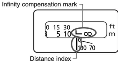
To compensate for shifting of the infinity focus point that results from changes in temperature. The infinity position at normal temperature is the point at which the vertical line of the L mark is aligned with the distance indicator on the distance scale.
