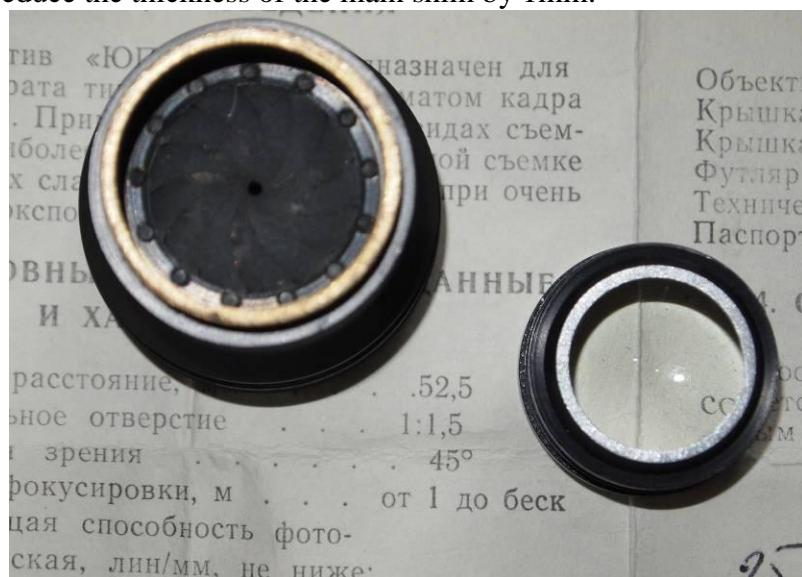
It is best to remove the glass from the main fixture. A spanner is required to remove the name ring and the retaining ring for the front triplet. The front triplet fits in very snugly, and pushing from the back through the aperture might be required. I use lens cleaning paper against the glass.
