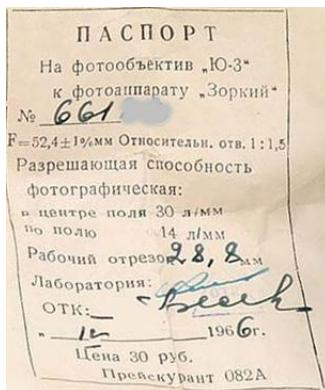
The focal length is given as  $52.4 \pm 1\%$ . That gives a range of about 51.9mm to 52.9mm. Those on the short end of the range will work well on a Leica. The average will work well once the main shim is adjusted, and those on the upper end will require the focal length to be reduced and then the main shim to be adjusted.
