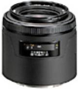
With an angle of view of 64 degrees, this lens is equivalent to a 34mm lens in 35mm format. With minimal perspective change, it produces the most natural image of all the wide angle lenses. A floating element mechanism improves resolution at the periphery in close-ups, for image sharpness all the way out to infinity. This lens is suitable for a wide range of situations, from general photography to scenics. It is designed to provide the feel of a standard lens with a slight wide angle effect.
