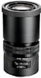
With an angle of view of 19 degrees, this lens is equivalent to a 130mm lens in 35mm format. Its natural focusing effect suppresses the foreshortening typical of telephotos while still isolating the subject. Excellent for a wide range of situations, and particularly for portraits. Super low-dispersion glass assures good contrast even for close-ups. The internal focusing mechanism makes handling easier, with no change in the balance between overall lens length and weight.
