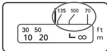
The infrared index corrects the focus setting when using monochrome infrared film. Focus on the subject manually, then adjust the distance setting by moving the focusing ring to the corresponding infrared index mark.
