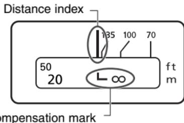
To compensate for shifting of the infinity focus point that results from changes in temperature. The infinity position at normal temperature is the point at which the vertical line of the L mark is aligned with the distance indicator on the distance scale.
