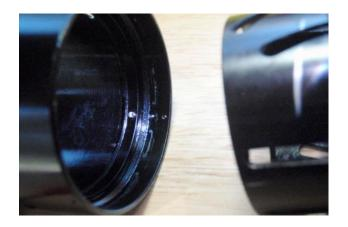
Left photo shows inside of cam ring, and the shoulder, which is where the 2<sup>nd</sup> and 3<sup>rd</sup> lens groups go. Right photo (left side) shows inside of zoom ring, and one of the two stops, and the grooves and shoulders for the proper alignment of the cam ring against those shoulders, before re-installing the retainer ring for the cam ring. Fine threads for the retaining ring for the cam ring are there as well.
