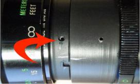
slide the rear mount assembly away from the rest of the lens. Also now slide the focal length indicator ring and the focusing distance ring off the lens – they come off easily. On one of my lenses, one of the 3 screws simply spun in its hole; using gravity it fell out. Appears the problem was stripped threads in the hole.
