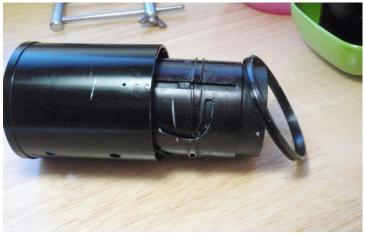
carefully cleaned, and some grease applied to it, as well with the threads into which it screws – these are in the zoom ring. The purpose being to make reassembly a little easier, and to make any future disassembly less difficult than it was. See also the pictures in the reassembly section, as this needed careful attention.
