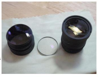
lens group was disassembled and cleaned, and reassembled onto the diaphragm assembly. What is the point of a mechanically good lens with hazy or oily glass? The goal here is clean and bright glass when everything is re-assembled, for those great pictures you'll be taking.
