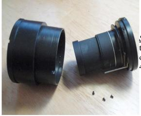
**Step #4.** Now remove the 3 screws connecting the two parts shown in photo left. Diaphragm blades are on right side of photo left. That part also includes the 4<sup>th</sup> (rear) lens group.
