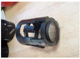
7. Be sure to install the zoom ring <u>before</u> installing the cam ring and 2nd and 3rd lens groups, and their associated screws and roller shafts and rollers. There are shoulders and grooves inside the zoom ring against which the cam ring rides, so the zoom ring must go on before cam ring.
