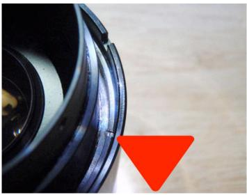
Note: my spanner wrench tips would not fit far enough in to reach the slots here. So I held, at an angle, a flat screwdriver in the notch, and gently, with a small hammer and repeated hammer taps and the screwdriver held about at a 45 degree angle, drove the notch with the flat screwdriver, with the lens on a table held by hand from turning by another person. Unscrewed this cam retaining ring that way; this is not recommended in any way and I should have avoided it.
