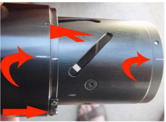
connecting that retaining ring to the outer helicoid; top arrow points to one of those 3 screws in the outer helicoid. The two curved arrows also point to scribe marks that line up in three parts – the outer helicoid, the outer helicoid retaining ring, and the inner helicoid – while they remain in the "full counterclockwise viewed from lens rear" position. This is the fully retracted or "bottomed" position.
