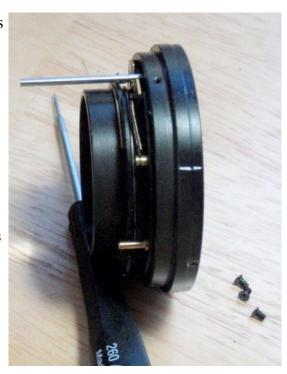
old grease from the helicoids and other parts, and re-lubricate with a good synthetic grease having a wide temperature range. I'm satisfied with the end result.
