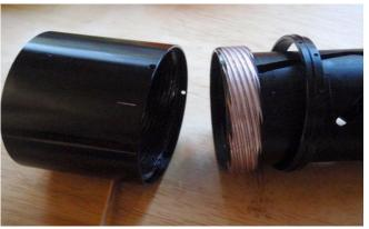
Also, when separating the two helicoids, at the place where they finally separate, put a mark (say, a white dot big enough to see easily) anywhere on one helicoid and another similar mark directly opposite on the other helicoid. Then, upon reassembly, start mating the helicoids where those two white dots are opposite each other. Saves time. And when in the "full counterclockwise viewed from lens rear" position, the helicoid scribe lines should line up as shown in the photo with red arrows.
