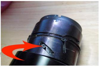
tweezers or another way to get the 4 roller shafts and rollers out of the slots. Also take out the other 3 screws in the cam ring slots.
