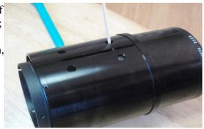
Suppose you forgot to put one of the metal tabs on before installing the cam ring and its retaining ring, so you can't put the metal tab in through the back. It is possible to maneuver the metal tab through one of the round holes in zoom ring, and then maneuver the metal tab into place on the outer helicoid retaining ring with gravity and pointed tools.
