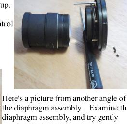
Here's a picture from another angle of the diaphragm assembly. Examine the diaphragm assembly, and try gently moving the levers that move the aperture blades. Try to gently work the aperture blades open and closed, with the lever (sometimes called the "blade operating lever") that has a spring attached to it; red arrow points to it If the blades don't move, maybe the cam on the other lever (sometimes called the "aperture cam ring") is holding the blades open; curved red arrow points to
