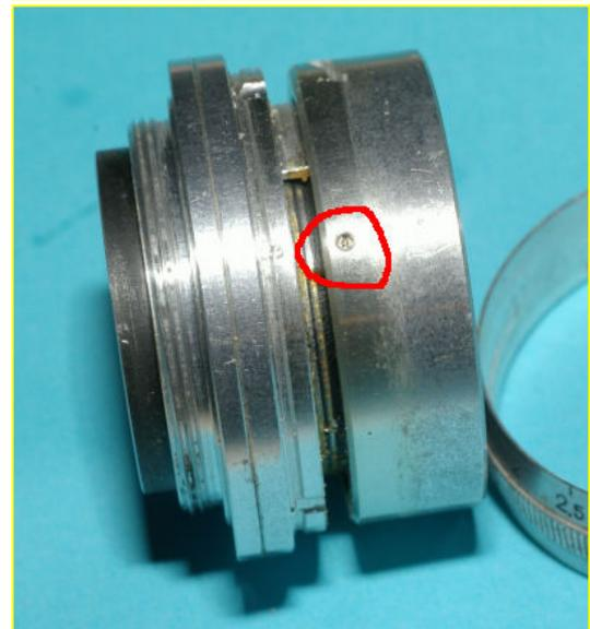
Remove the 3 screws around the keeper ring on the bottom and lift of the ring.
