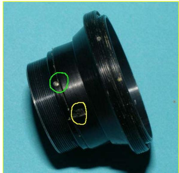
Both parts can now be carefully cleaned. To re-lube this part, I use a lithium-based grease that is a bit thicker than the silicon based grease used on the helix. The arrow shows the important part. It is this rubbing on the main body that gives the diaphragm it's "feel". By using a thicker grease, I find the ring is smooth to turn but less likely to get knocked out of place whilst focussing. Use a little to start with and add more till you get the right feel for you.
