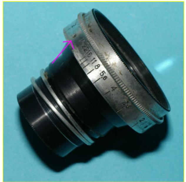
Now undo the 2 screws around the top of the lens just below the front surround. In this case, they were buried in the grease so you may need to hunt for them. The front nameplate ring can now be unscrewed.
