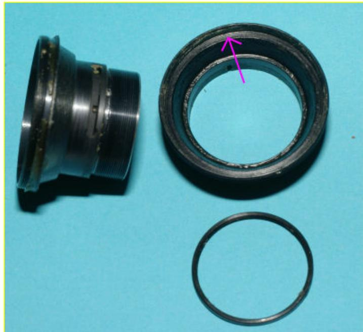
Reassembly is the reverse procedure. When you replace the outer diaphragm ring, leave the 3 screws slightly slack. You will need to adjust this once the lens unit is replaced on the focus unit to get the index mark in the right place.
