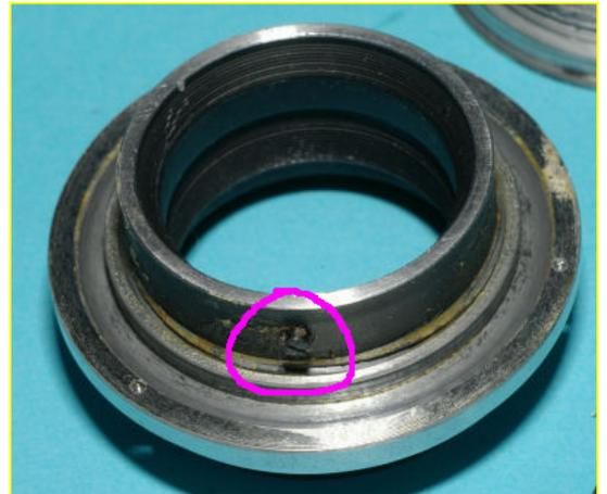
Note how this looks. With the helix unit inserted correctly, the top of the body ring is nearly touching the rim of the helix unit. Only one start position of the 4 possible will look like this so when you re-assemble refer to this picture. Separate the 2 parts, clean re-grease and reassemble in the reverse order. Place this unit on a camera and move it to infinity and check that the RF is also on infinity. If not, the helix is in the wrong place.
