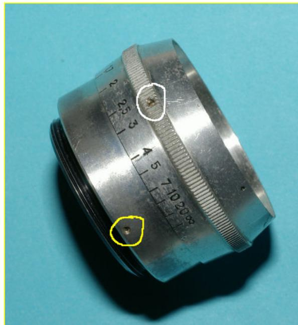
With the lens set at the close focus point, note how the 2 stops screws almost touch either face. Remember this, as you will when you reassemble to get the helix in the right place. Unscrew the helix slightly so you can get at the lower screw (arrowed in yellow) and remove it. You can now remove the helix unit.
