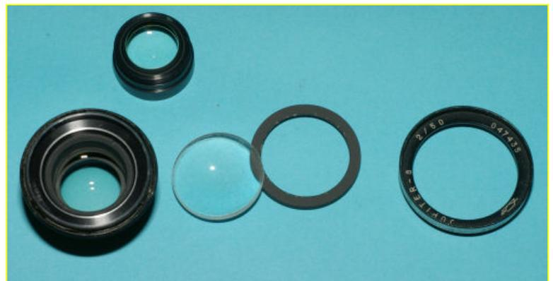
The second lens group should now also come out although in some cases it may be a bit stiff and need a gentle prod from the back. Note the 2 cut-outs for a lens spanner in the picture. There is no need to do anything here unless you want to slit the second group to clean the glass. This is best done with the group removed.
