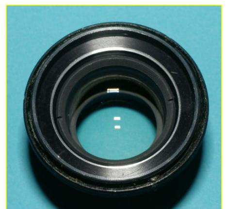
If the diaphragm is dirty, you can now clean it with a cotton bud and some Ronsonol lighter fluid. To re-lube the ring, first remove the index pin marked here in yellow. Next remove the lock ring screw shown in green. The ring will now unscrew and the two halves can be separated.
