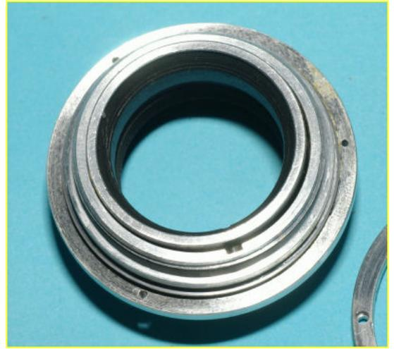
Remove the guide pin. If you decide to remove the stop pin as well remember that the guide pin is the shorter of the two.
