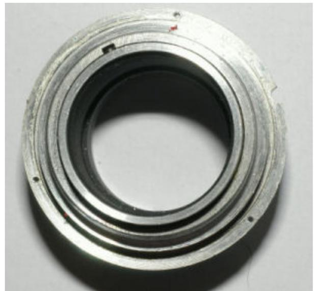
Have a good look at the focus helix. It has one of four start positions and it is important to get the right one or the lens will not focus correctly. You may want to mark the position as shown here by the yellow circle. If not, note how the alloy body ring almost touches the focus helix as it touches the limit pin. Having done that, remove both the limit pin and the guide pin shown in the photo. Note that the guide pin is slightly shorter than the limit pin.
