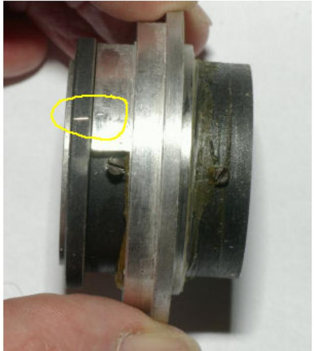
Unscrew the two rings. Note the old decayed grease. Carefully de-grease all the 4 components. (Focus helix, main body ring, lens mount and locking ring).
