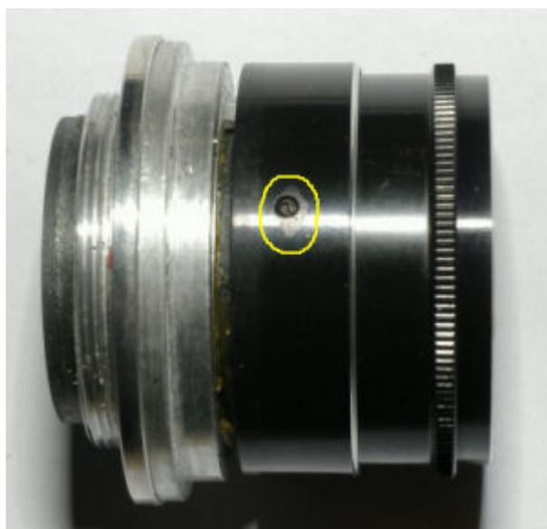
Using a pair of ground pliers or a lens spanner, remove the rear-retaining ring and unscrew the ring. As you start to unscrew it, the lens unit will become loose so you will need to support it from the front. Once it is slack, you should be able to unscrew the lens unit from the front. Put it safe to one side.
