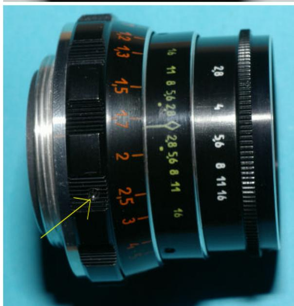
Either slacken off or remove this screw. It is the one directly opposite the depth of field scale.
