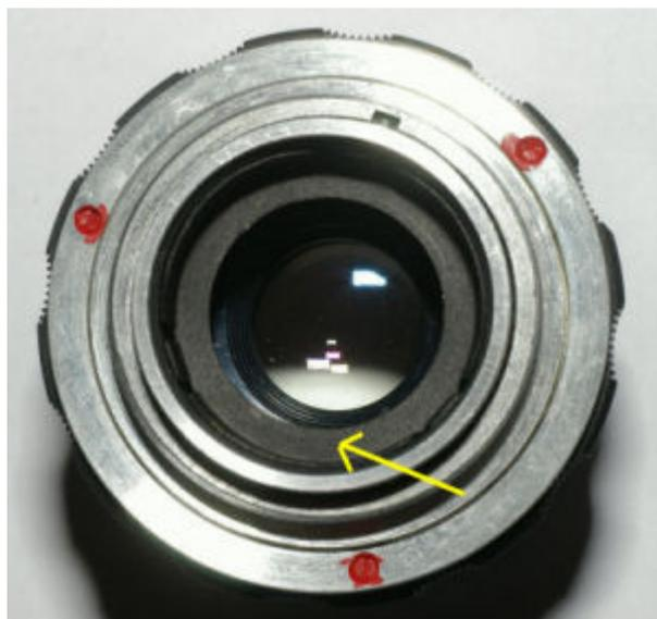
Remove the 3 screws around the focus ring and remove the ring.
