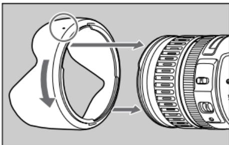
The EW-78B II lens hood can keep unwanted light out of the lens, and also protects the lens from rain, snow, and dust. To attach the hood, align the hood's attachment position mark with the red dot on the front of the lens, then turn the hood in the direction of the arrow until the lens's red dot is aligned with the hood's stop position mark. The hood can be reverse-mounted on the lens for storage.
