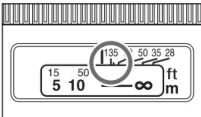
The infrared index corrects the focus setting when using monochrome infrared film.
