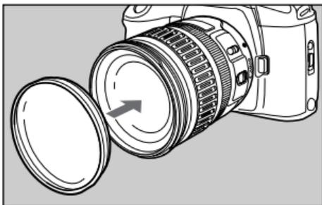
You can attach filters to the filter mounting thread on the front of the lens.
