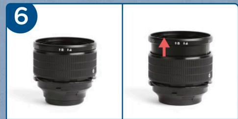
**EN** The Edge 80 has a built-in close focus feature at the front of the optic. Pull the front of the optic forward to focus closer. In this position, minimum focus is 19". Tilted, minimum focus is 14-15".
