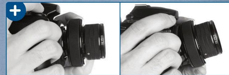
**EN** Point your lens body straight ahead for your first few shots. Everything in the same plane will be in focus – just as if you were using a standard lens. Tilt the lens body left or right for a vertical slice of focus, up or down for a horizontal slice and diagonal for a diagonal slice. Re-adjust focus as needed.
