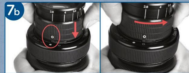
**EN** Align the hollow dot on the optic with the solid dot on the lens body. Firmly grip with fingers positioned as shown on the Aperture Ring. Push down and turn counter clockwise until the hollow dot on the optic and the hollow dot on the lens body align.
