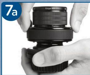
**EN** To remove your Edge 80 Optic, first tighten the Tension Ring at the base of the lens body. Firmly grip with fingers positioned as shown on the Aperture Ring. Push down and turn counter clockwise until the hollow dot on the optic and the hollow dot on the lens body align.
