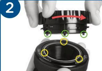
**EN** Insert the 3 teeth of the Optic Swap Tool into the 3 notches. Push down and turn counter clockwise to unlock. Turn the lens body upside down.
