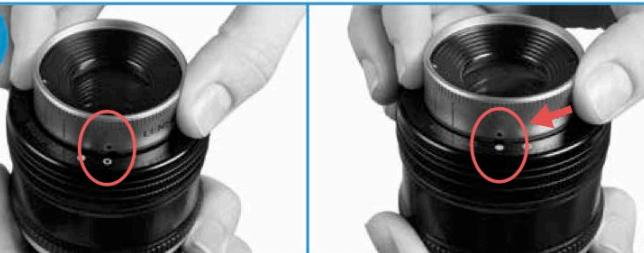
**EN** Next, align the Optic's white line and solid dot with the hollow dot on your lens body as you insert the Optic. To lock, turn the Twist 60 clockwise until the solid dot on the Optic and the solid dot on the lens body align.
