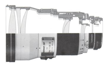
●Focal Length: 300mm ●Maximum Aperture: F/2.8 ●Minimum Aperture: F/32 ●Angle of View: 8° ●Lens Construction: 7 elements, 6 groups ●Coating: BBAR multi-layer coating ●Minimum Object Distance: 3.0 meters (9.8 feet) ●Filter Size: 43mm (rear) 112mm (front) ●Mount System: Adaptall-2 interchangeable mount system ●Overall Length: 203.5mm (8 inches) w/mount for Nikon ●Diameter: 117.5mm (4.6 inches) ●Weight: 2,071 grams (73 oz.) ●Hood: Bayonet-type, supplied with the lens
