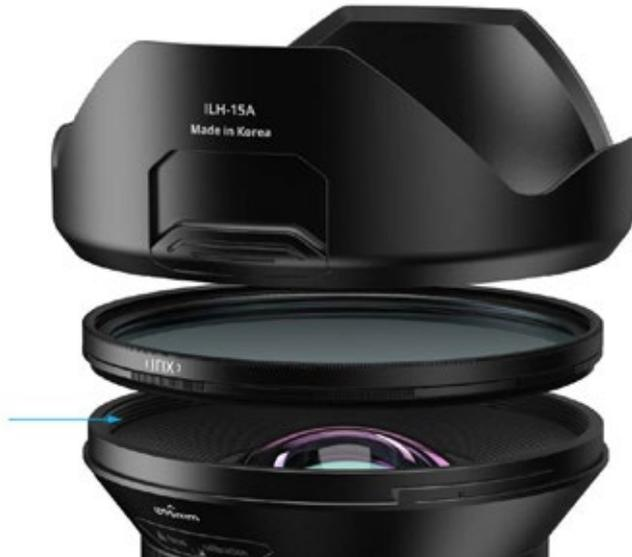
Your Irix lens can accept 95 mm screw-in filters via the front threads. Due to the wide angle of view, the use of “slim” filters is advisable to prevent vignetting. Filters with a low profile of 5.3 mm or less are recommended. Stacking multiple filters may also cause vignetting.
