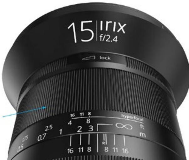
The focusing ring moves the internal focusing elements of the lens to achieve the desired focal point. You can focus visually while looking at your subject in the viewfinder or LCD screen or by using the distance, depth of field or hyperfocal scales on the lens barrel.
